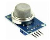
A gas sensor is a device which detects the presence or concentration of gases in the atmosphere. Based on the concentration of the gas the sensor produces a corresponding potential difference by changing the resistance of the material inside the sensor, which can be measured as output voltage. Based on this voltage value the type and concentration of the gas can be estimated.
