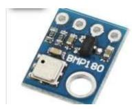
A pressure sensor is a device that measures the force applied on a surface per unit area and converts it into an electrical signal. These sensors are widely used in various applications across industries, including automotive, medical, industrial, and environmental monitoring. The key details about pressure sensors include the types, working principles, applications, and considerations.
